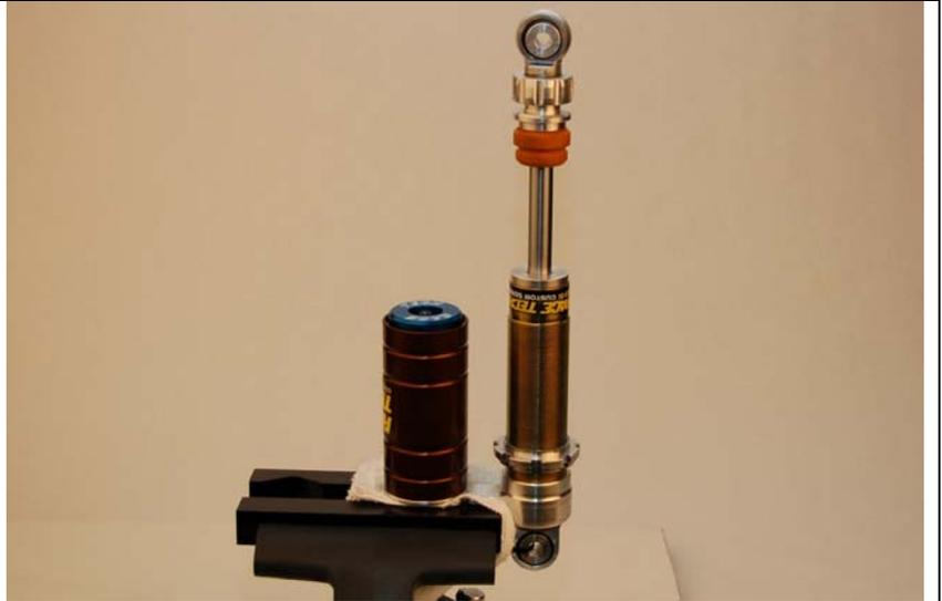
2. **Select the appropriate Bladder Adapter.** Insert the Adapter into the Reservoir and install the stock Bladder Cap Clip. Thread on the Adapter Plate (TSVM ABP70) and draw the Adapter up to the Clip. Then Attach the Control Head to the secured Adapter.
