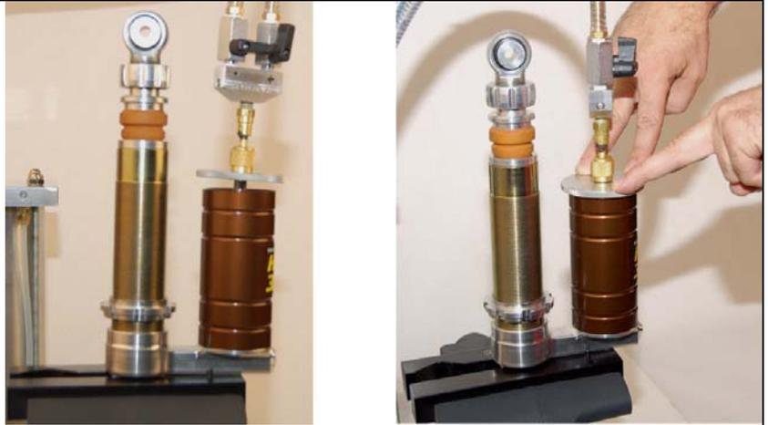
11. Disconnect the Control Head from the Adapter. Remove the clip and the Adapter.
