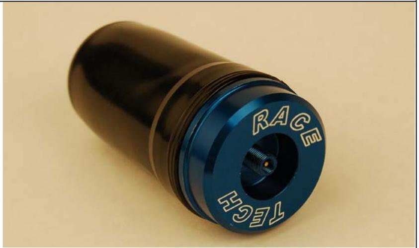
13. Insert the Clip, seat the Cap and pressurize the shock with nitrogen to the recommended setting.
