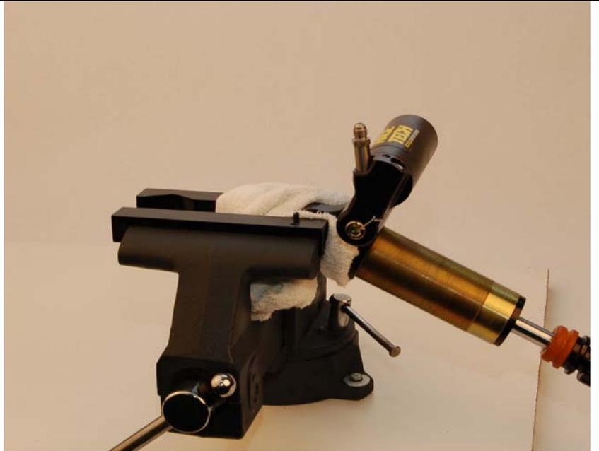
3. Loop the filler hose upward.
