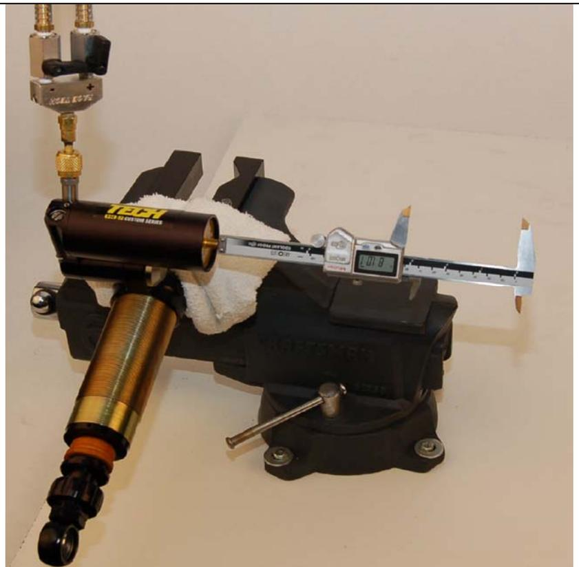
11. Disconnect the Control Head from the Adapter. Remove the Adapter. Replace the Bleed Port Screw and pressurize the shock to the recommended setting. Make sure any required o-rings are in place.
