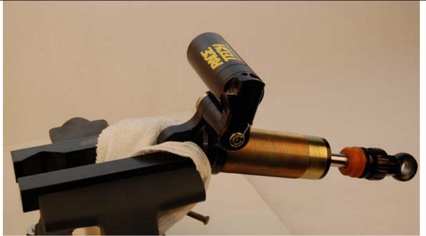
2. **Select the appropriate Adapter.** Remove the Bleed Screw and attach the Adapter to the Shock. Then attach the Control Head to the Adapter.
