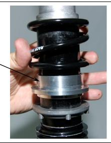
7. Install the new GBT (Go-Between) Collar. It MUST be installed with the long flange facing the Secondary Spring.
