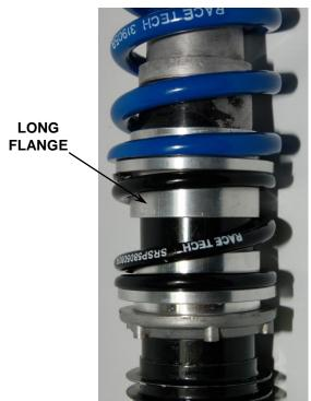
8. Install the Main Spring. Measure the overall length of the two springs together including the GBT. This is the Free Length. It will be used in setting the preload.
