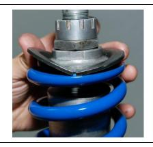
Preload is the amount the spring <u>set</u> is compressed from its Free (uninstalled) Length when it is installed on the shock.
