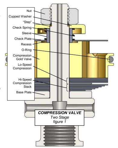
will not tighten down on the valving. This will cause incorrect operation or the nut will come off. This is a critical part of the installation. To get the proper total valve stack thickness you may need to place some of the original shims on the shaft just after the base plate. NOTE: Any shims added must be larger in diameter than the last shim in the stack. **Be sure the nut is fully engaging the threads!**
