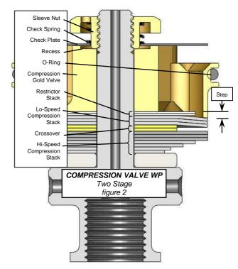
**The Restrictor Valving Stack serves 2 purposes.** First, its diameter can restrict the port size. Second, its thickness can create preload.
