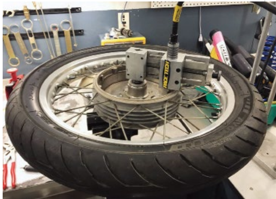
Race Tech's proprietary tool in place to machine the 1973 BMW R75/5 front drum.
