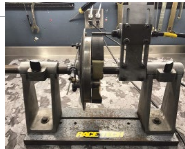
Brake backing plate with shoes jugged up on Race Tech's brake arcing tool to cut and match the profile of the shoes to the drum.
