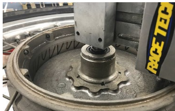
Black lines act as cutting guide; when they're gone, the drum's done.
