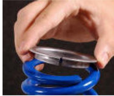
10. Insert the smaller of the two sizing collars into the larger. This will size the spring for the stock retaining collars.
