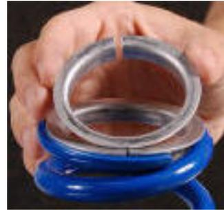
11. Measure the overall length of the two springs together including the GBT. This will be used in setting the preload.
