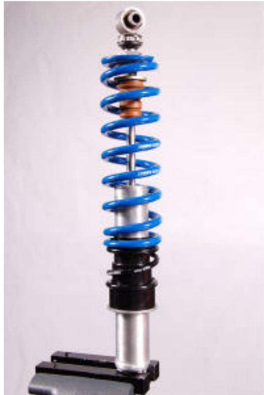
9. Install the larger of the split sizing collars into the spring. You will need to squeeze it slightly to make it fit.
