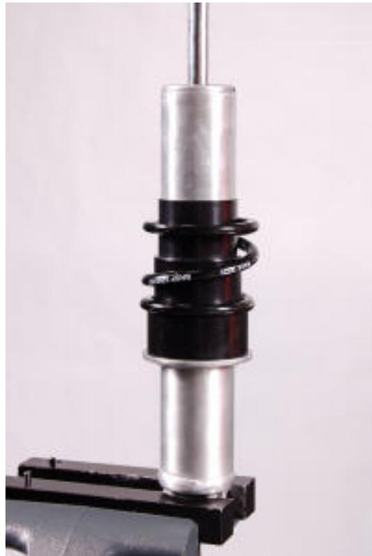
7. Install the new GBT (Go-Between) Collar on the stepped collar. It MUST be installed with its internal taper facing AWAY from the Secondary Spring. This means the smallest inner diameter on the GBT will hit the step on the Stepped Collar when in use. **THIS IS CRITICAL.**
