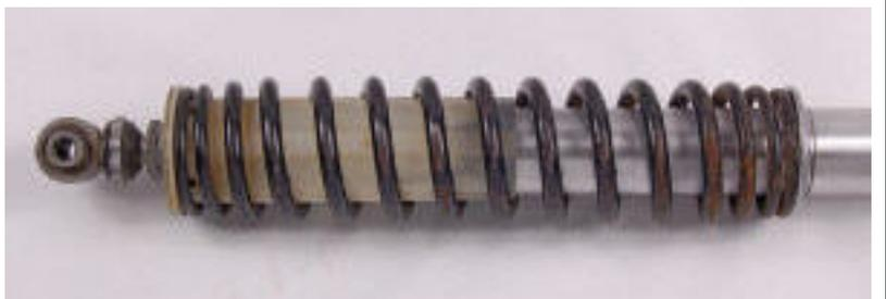
2. Loosen the locking nut. Back off the preload adjuster all the way and remove the spring retainer clips.
