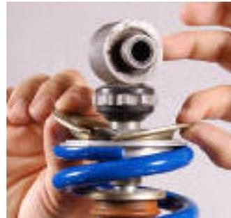
13. Screw in the preload adjuster until you achieve 8 to 10mm of initial preload. This is a good starting point for most riders when the main spring rate is correct. Tighten the Locking Nut. On some models you may have to reposition the wire clip on the body.
