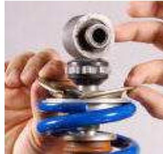
11. Screw in the preload adjuster until you achieve 7mm of initial preload. This is a good starting point for most riders. Tighten the Locking Nut.
