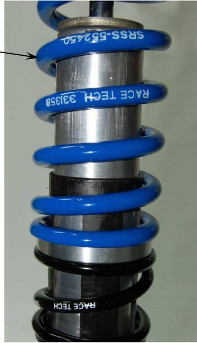
8. Install the sizing collar into the spring.
