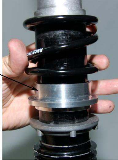
7. Install the new GBT (Go-Between) Collar. It MUST be installed with the long flange facing the Secondary Spring.
