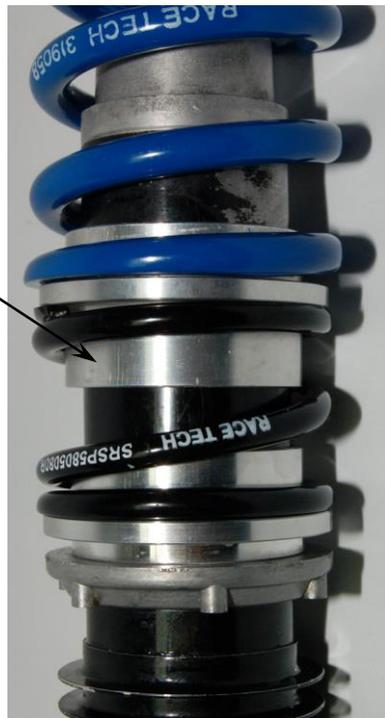
8. Install the Main Spring. Measure the overall length of the two springs together including the GBT. This is the Free Length. It will be used in setting the preload.
