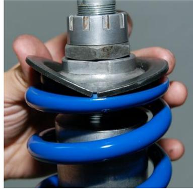
10. Preload is the amount the spring set is compressed from its Free (uninstalled) Length when it is installed on the shock. Be sure to measure the combined length of both springs.
