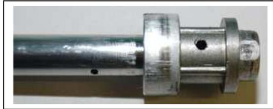
**KYB Closed Top Style Damping Rods Requires Machine Work on Lathe along with Gold Valve Adaptor:**
