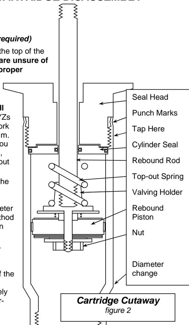
**CYLINDER SEAL INSTALLATION**
