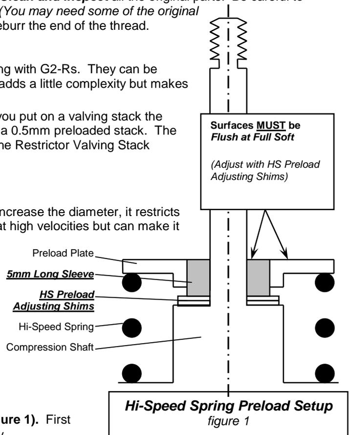
(counterclockwise). Install the Hi-Speed Spring, the **5mm long Sleeve**, and the Preload Plate. **Add HS Preload Adjusting shims (9mm od shims) until the top of the Preload Plate and the top of the Sleeve are equal (zero preload).**
