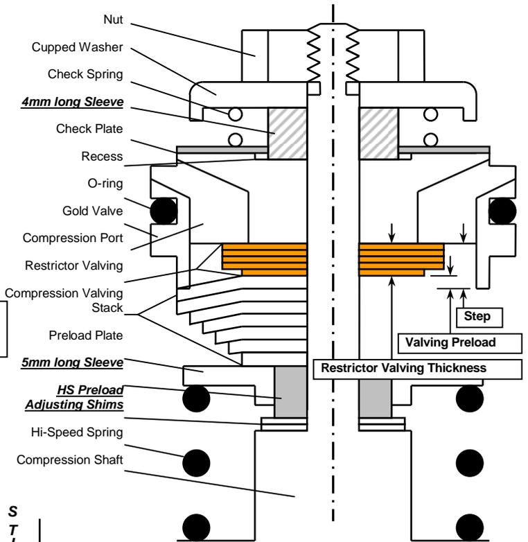
**G2-R Gold Valve Cutaway**
