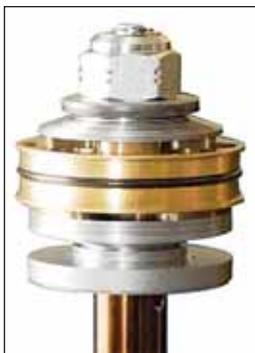
*This rebound separator valve, at left, and Gold Valve, above left, assemble on the shaft of the Suzuki's stock shock, below left. The separator keeps rebound damping adjustments from affecting compression damping.*
