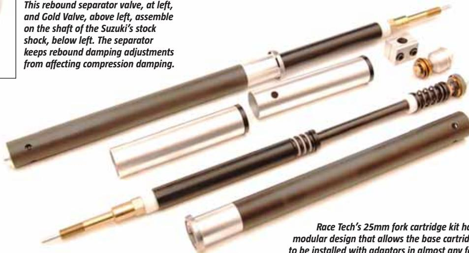
*Race Tech's 25mm fork cartridge kit has a modular design that allows the base cartridges to be installed with adaptors in almost any fork.*
