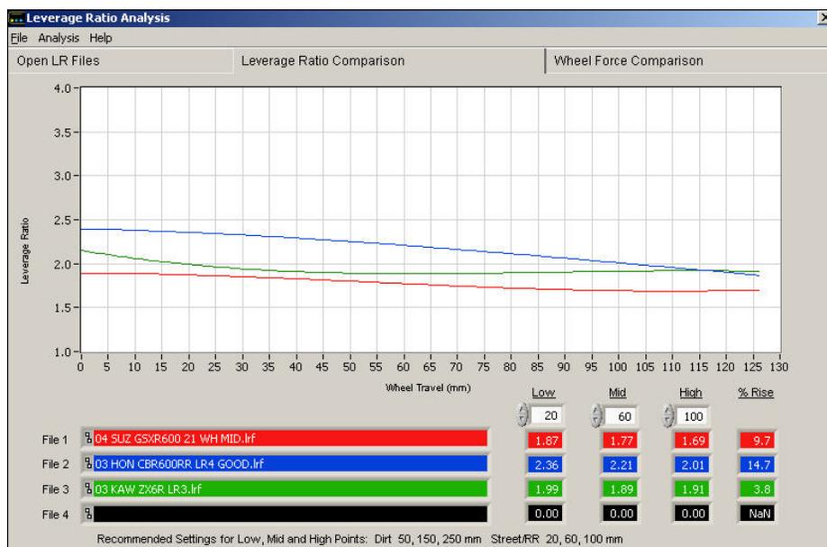
For example a 04 YZ 250 has a rise in rate of around 33% while a KX 250F has 15%. From experience this means the KX 250F will have more of a trade-off. It will be more difficult to get bottoming resistance while retaining plushness on the smaller bumps. Experience is the key.
