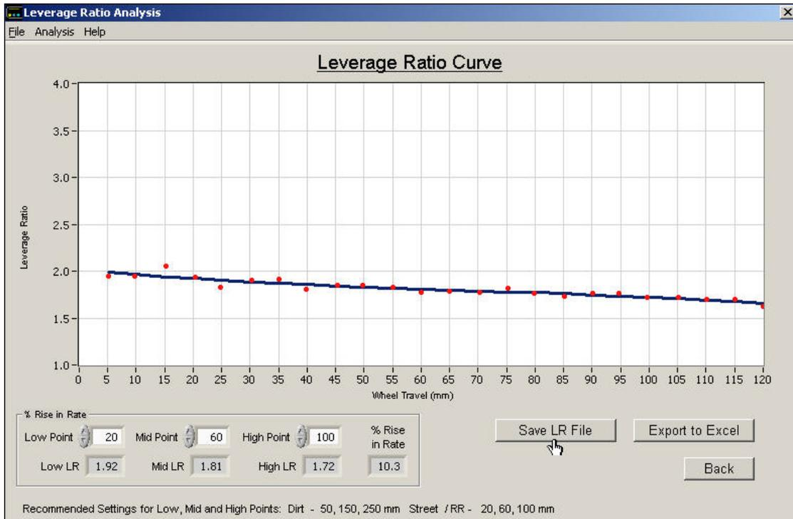
The Leverage Ratio curve is created from the Shock and Wheel data. The red dots are the “raw” Leverage Ratio points. The blue line is the calculated Leverage Ratio Curve.
