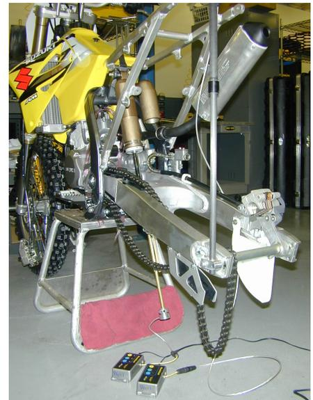
5. Align the LR Transducer with the shock. Extend the small Control Rod and hose clamp it to the Shock Body. Align the LR Transducer Tube, the Control Rod, and the shock shaft. You may have to bend or twist the aluminum mounting strap or flip the clamp to get a good angle. If it is slightly misaligned it may be OK. **Make sure there is always clearance and there is no contact with the linkage as you move the swingarm through its entire travel. Adjust as necessary.**
