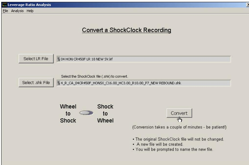
Select the Leverage Ratio File (.LRF) you want to use. Then select the ShockClock file you want to convert. Select “Wheel to Shock” if the ShockClock recording was taken at the Wheel and you want **“as if recorded at the Shock”**.
