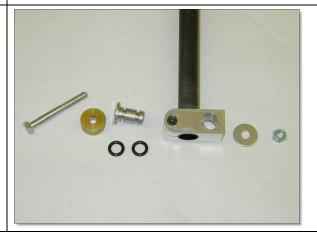
This photo shows the completed assembly ready to be inserted into the axle.
