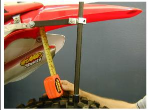
Measure the travel of the transducer as it is mounted. Make sure the exposed transducer travel is greater than the wheel travel.
