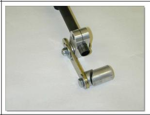
Locate the clamp as close to the top of the swingarm as possible without hitting.
