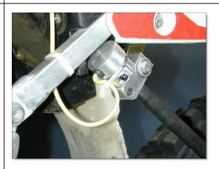
It's important the rider doesn't hit it with his boot while riding. Mounting on the inside allows the number plate to be reinstalled for testing. Use washers as necessary to space the number plate out or the Transducer in.
