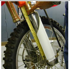
Measure the travel of the transducer as it is mounted. Make sure the exposed transducer travel is greater than the wheel travel.
