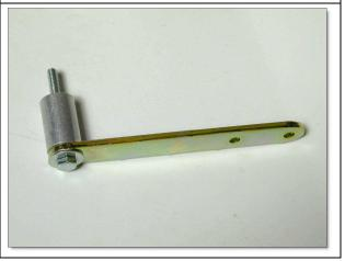
Typical installation is on the left side of the bike (the side without the pipe). Find a side panel, fender or seat mount and attach the upper bracket horizontally (you may need to remove the side panel. Tighten securely.
