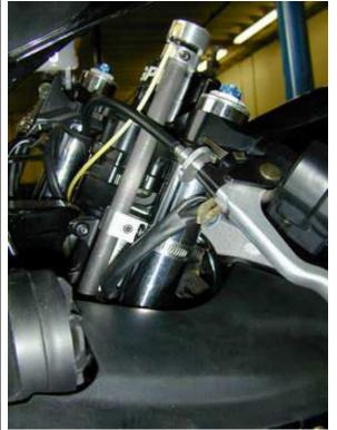
Notice the Remote Record Switch mounted on the Clutch perch. This Switch comes with the Pro kit and allows remote control of two ShockClocks.
