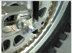
The complete rear assembly should have the transducer tube mounted approximately vertically when viewed from all angles as shown.
