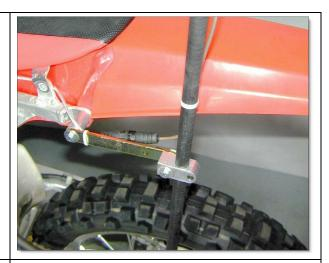
Zip-tie the transducer cable securely then route it across the bike frame to the handlebar mounted ShockClock. Make sure the cable is not stretched when the bars are turned.
