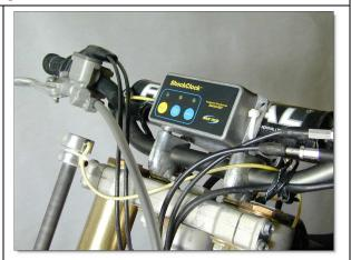
ShockClock be mounted metal-to-metal or damage could result.
