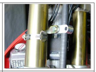
You may be able to mount the upper transducer bracket on the lower triple clamp pinch bolts.
